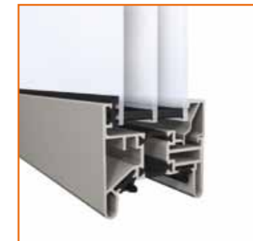
Panorama door 60 mm Triple Plexiglas Optical 40 mm (4-14.75-2.5-14.75-4 mm)
